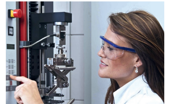
Tensile testing machine to check tensile strength of elastomers and plastics in contact with our lubricants.
